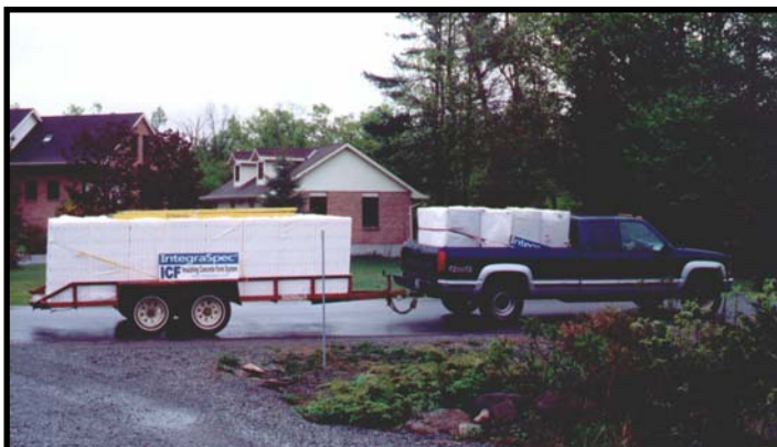
Shipment for 1200 ft 2 foundation, eight units high
