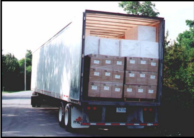
53' trailer holding 7200 ft 2 finished wall space
