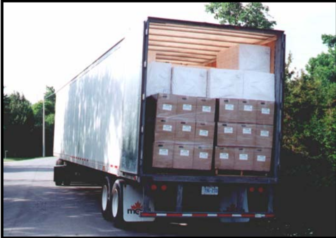
53' trailer holding 7200 ft 2 finished wall space
