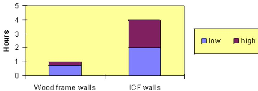
This has been confirmed in so-called “fire-wall” tests. In these tests ICF walls were subjected to continuous gas flames and temperatures of up to 2000°F for as long as 4 hours. None of the ICF walls ever failed structurally. All of the ICFs tested were of the “flat” or “uninterrupted grid” type, having no significant breaks in the concrete layer. In contrast, wood frame walls typically collapse in an hour or less.
