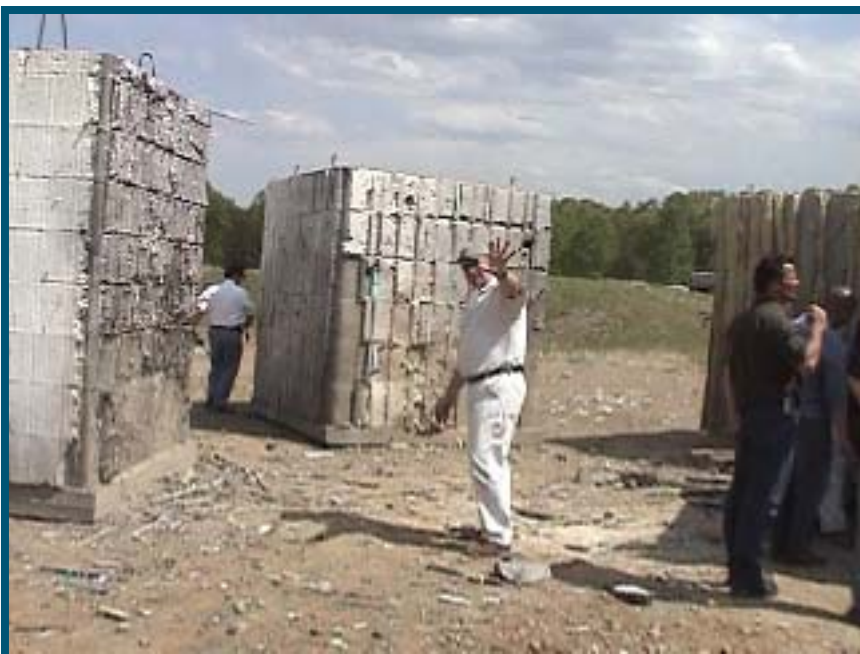
IntegraSpec’s box (on the left) after the blast test
